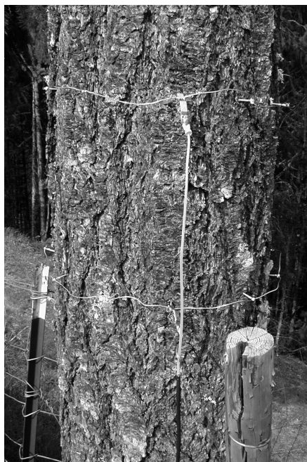
Figure 1 — Impedance measurement on a Douglas fir tree.
